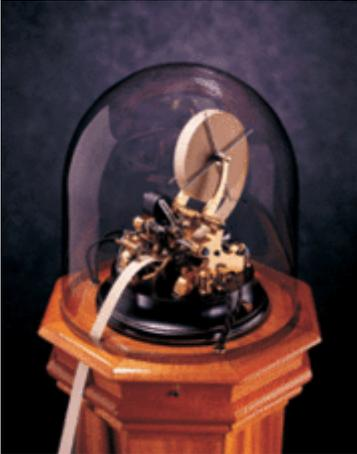
**A stock ticker converted something similar to Morse code into a printed strip of paper with a stock's symbol and trade information such as price.** The thin strip of paper was referred to as tape, and the ticking sound made by the machine gave it the name ticker tape. Such devices were used until the 1960's when they were replaced by computers. You can
